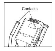
your heart rate, hold the handgrip pulse sensor with your palms resting against the metal contacts. Avoid moving your hands or gripping the contacts tightly.
